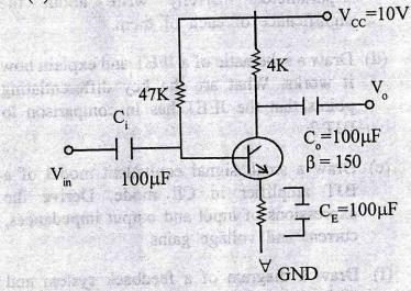
Find the voltage gain of the circuit.
